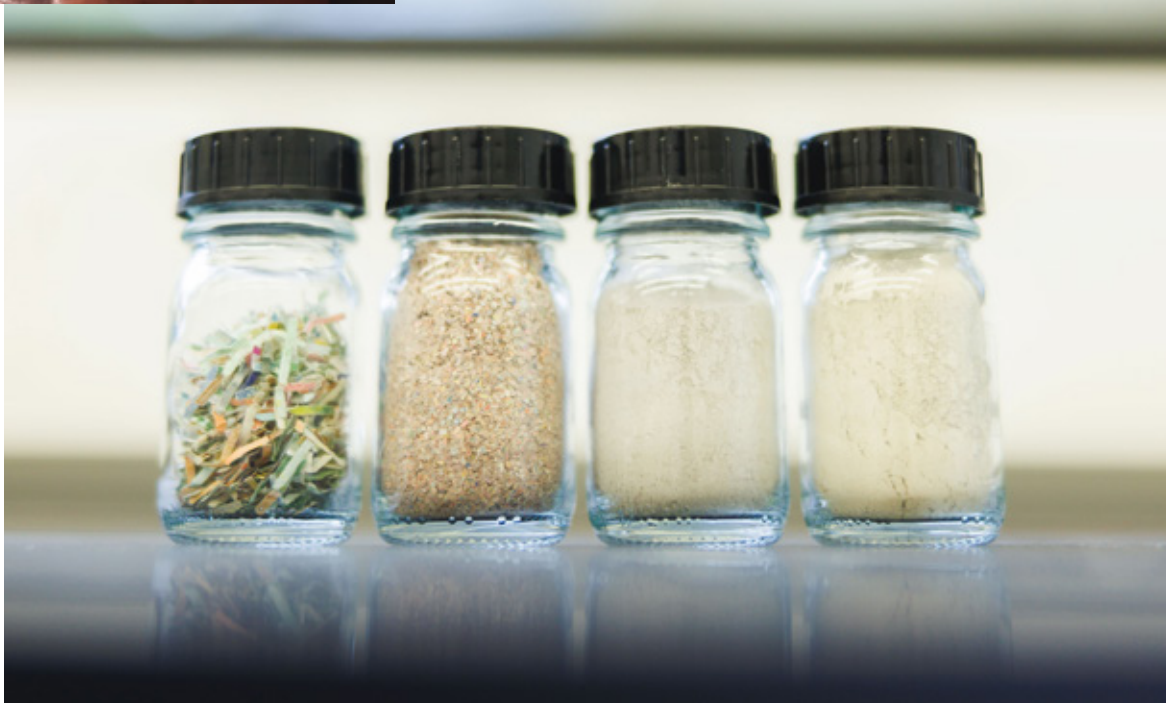
The lanthanide europium can also be found in old banknotes. The bacteria in Professor Daumann's laboratory are given shredded banknotes (far left; adjacent: ground to powder and in the form of ashes) to eat. They extract the coveted elements in the process.
