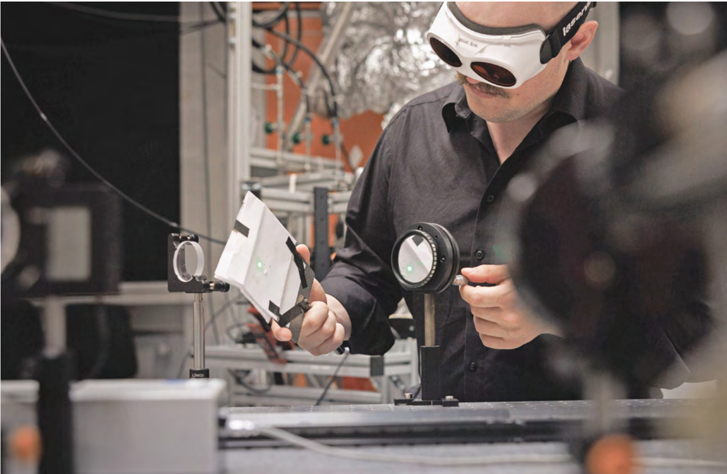
Erik Wüst, a doctoral researcher whose supervisor is Professor Brezinsek, fine-tuning the optics for the picosecond laser plasma spectroscopy.
