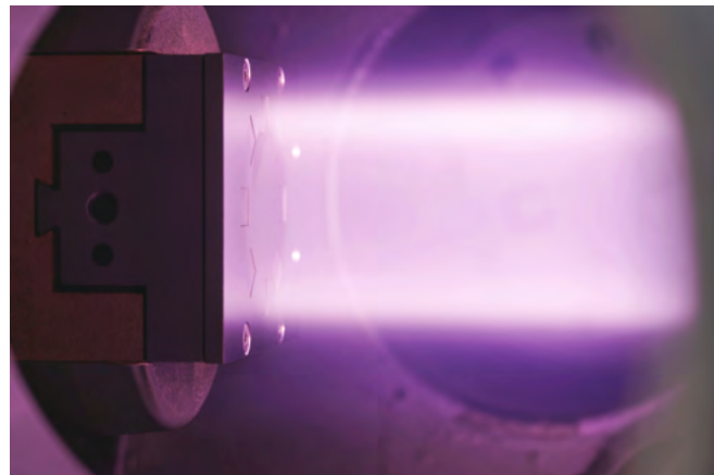
The deuterium plasma strikes a plate holding samples arranged in a ring (left). The aim of this is to examine how the wall material in a future reactor will respond to plasma bombardment.
